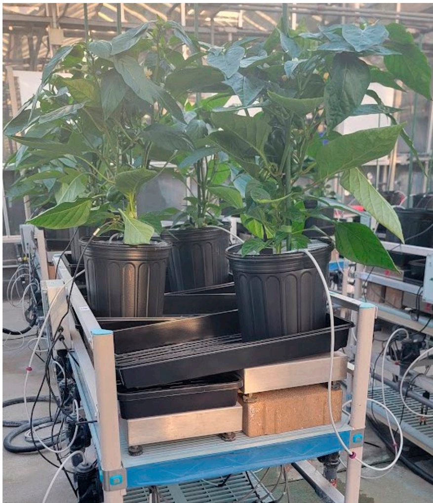
Fig. 1. Greenhouse bell pepper plants grown in individual containers on an automated gravimetric irrigation platform equipped with load cells, irrigation tubing, and drainage collection trays for continuous monitoring of plant water use and controlled irrigation delivery.
